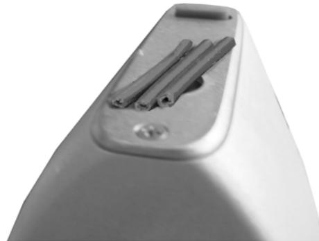
**Figure 1-4. Wire insulation cut into strands.**
