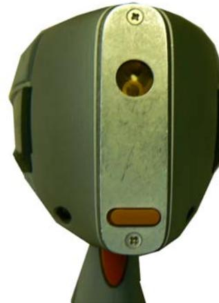
Figure 2-6. View of Face Plate and Kapton Window
