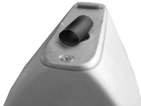
**Figure 1-6. Incorrect Way to Measure Heat Shrink Tubing**
