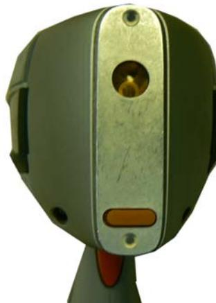
**Figure 2-8. Fitting Face Plate over Proximity Button**
