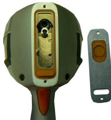
Figure 2-7. Face Plate Removed showing Kapton Window on Reverse
