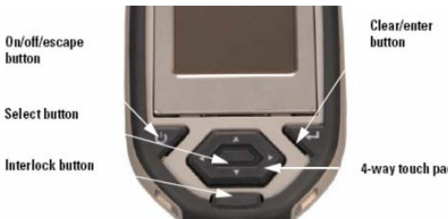
**Figure 1-29. The Control Buttons for the XL3**
