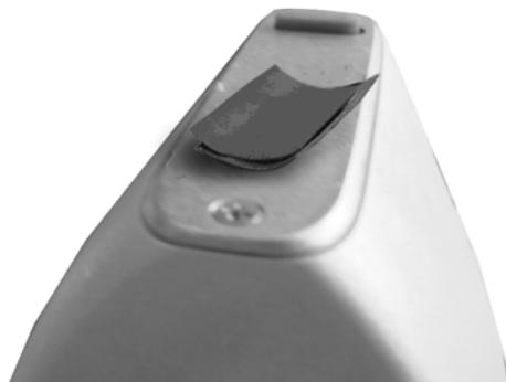
**Figure 1-7. Correct Way to Measure Heat Shrink Tubing**
