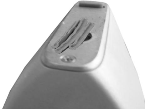
**Figure 1-5. PVC wire insulation with conductor removed**
