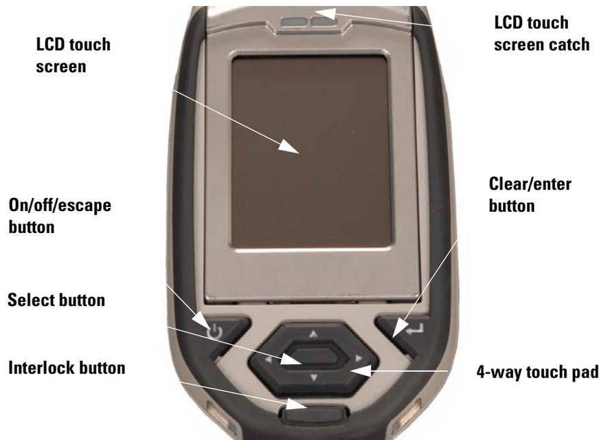
**Figure 0-2. The Control Panel**
