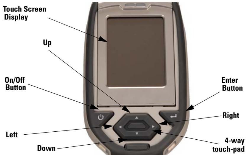
**Figure 1-33. The Control Panel**
