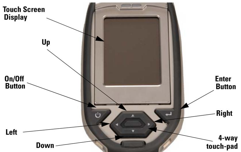
**Figure 1-10. The Control Panel**
